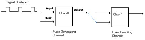
NOTE: the signal connected to the input of counter channel 0 will be routed to the input of counter channel 1 internal to the AM9513A chip. This is a special feature of the AM9513A chip.
